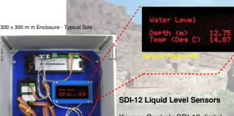
Keynes Controls SDI-12 digital network encapsulated water level sensor.
