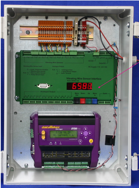
Example VibWire-108 application using the DT80 Logger.
