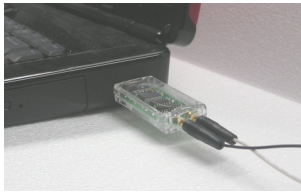
USB media converter installed into a Notebook/Laptop PC.
