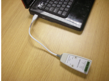
Image above shows the USB-RS485-Pro media converter connected to a Windows
