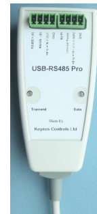
Fig 30 - USB-RS485-Pro connection to a single I-P-I RS485 model sensor
