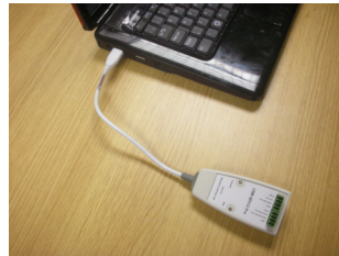
Fig 28 - USB-RS485-Pro media converter installed on a laptop computer.
