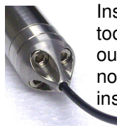
Fibre Optic cable connected to the AquaBAT Unit
