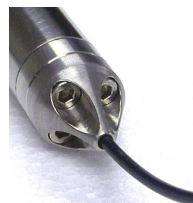
Fibre Optic cable connected to the AquaBat Unit
